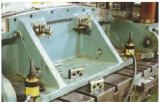
图中使用两个RCH-6050液压油缸来 夹住这一大型模具，通过空心柱塞来 定模槽栓。 Two RCH-6050 cylinders are used here to clamp this large die. The hollow plunger allows fixing of the slot bolt.
